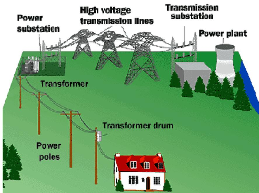
The advantage of ac over dc is that in ac, voltage can be **changed whenever is needed**. At a power plant at Eskom the terminal voltage ranges from 115 kV to 650 kV. Power substation reduces it to 7.2 kV. The transformer in the city reduces it further to 230 V as required by household appliances.
