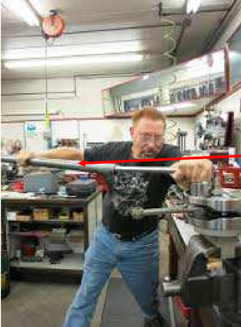
A mechanic is loosening a tight nut. He could ask a colleague to assist him exerting more force. That will increase a turning effect or a torque on a nut. Instead, he decided to use an extension pipe to increase the lever arm ( $r$ ) and thereby increasing a torque ( $\tau$ ).
