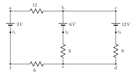
(a) For the circuit shown above, with the directions of the currents chosen as shown, obtain three equations from which  $i_1$ ,  $i_2$  and  $i_3$  can be determined. (DO NOT SOLVE FOR  $i_1$ ,  $i_2$ , and  $i_3$ .)
