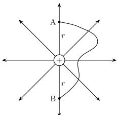
3. Two charges, Q and -2Q, are located at points A and B as shown in the diagram below. Circle the point(s) on the line joining the two charges, which correspond most closely to the positions where the electric potential is zero.
