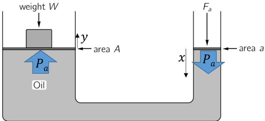
Consider applying a force  $F_a$  on the left cylinder in the diagram, over the area  $a$ , in an attempt to lift an object of weight  $W$ . The pressure exerted on this cylinder is given by
